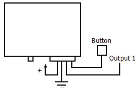
Remuc can be configured to control vehicle ventilation. In this case connect Output 1 (PIN10) or Output 2 (PIN11) to car ventilation control. This enables user to control ventilation either simultaneously with or separately from heating.
