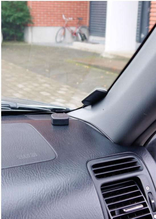
The install height of the antenna plays a great role in getting the best possible signal reception. Generally, the higher the antenna is, the better is the reception. Bottom edge of the windshield is a good example.
