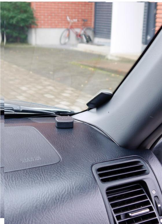
The install height of the antenna plays a great role in getting the best possible signal reception. Generally, the higher the antenna is, the better is the reception. Bottom edge of the windshield is a good example.
