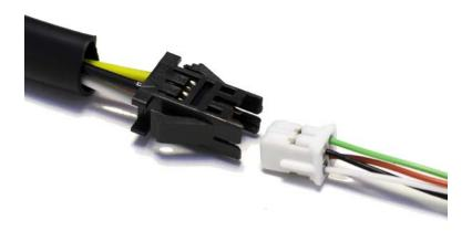
If the delivered GPS receiver model doesn't have the shown connector, you need to connect the wires manually into the 16-pin Remuc connector. Pay attention to the Wire contact orientation when inserting them into Remuc connector. Wire contact going in the plug must be in correct orientation, otherwise breakage may occur.
